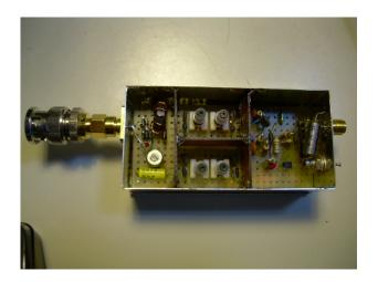
INPUT ---> OUTPUT: in 10MHz +5dBm out 100MHz +10dBm. Signal to harmonics and sub-harmonics ratio more than 60 dB.
