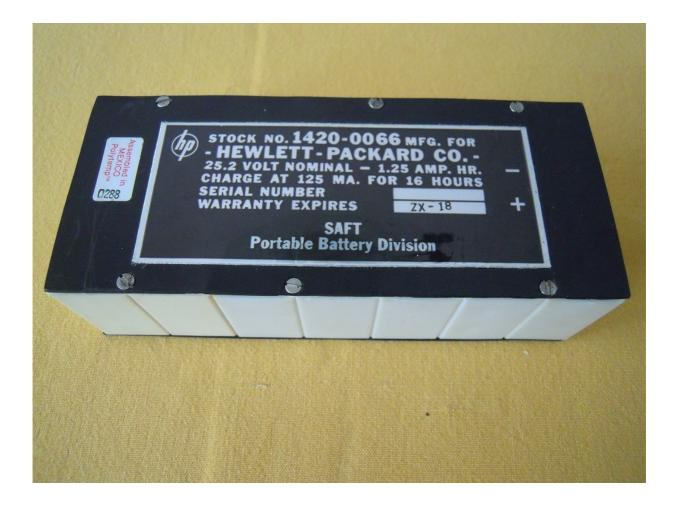
The battery pack is housed in a plastic box in three row 7 battery each for a total of 21 single Nicad 1.2 Volt 1.25 Amp. Hr. The serial connection of the elements provides a voltage rating of 25.2 Volts.
